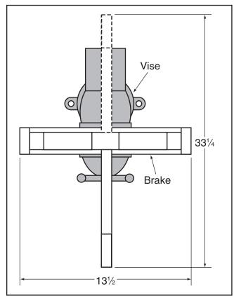
Figure 2. Minimum working clearances.
